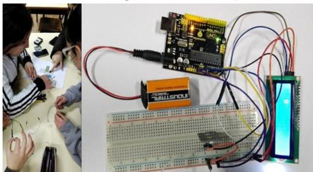
Figure 2. Assembly process and final result for the sensor that shows in real time the UV index.
