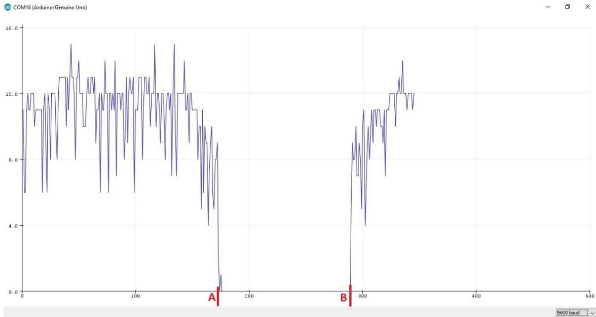
Figure 6. Graph representing the intensity of the UV radiation over time, with point A being the moment when the sunglasses were placed in front of the sensor and point B the moment when sunglasses were removed.
